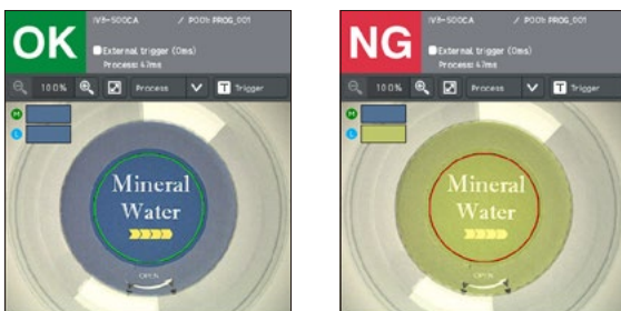
(Colour-based cap difference check)
