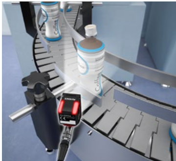
Cap tightening check
