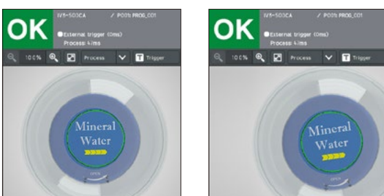
(Mark presence detection with rotational correction)
