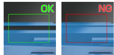
Photocopying machine screw check
