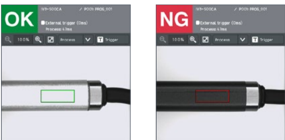
(Type-based difference check of metal components)
