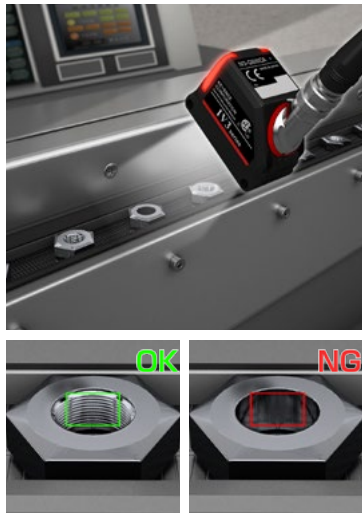
Processing-based metal component difference check
