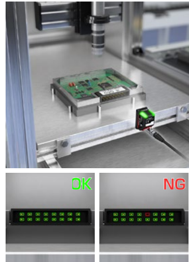
Connector pin breakage check
