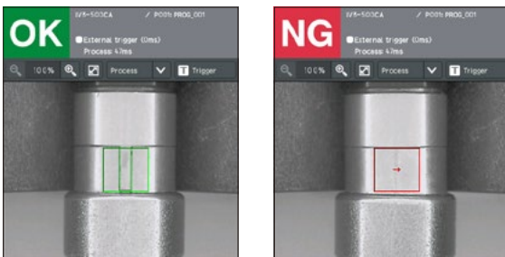
(Type-based difference check of metal components)
