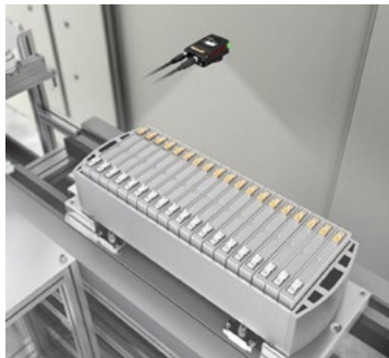
Lithium-ion battery orientation check
