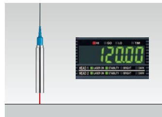
When the sensor is installed perpendicular to the target: A large amount of reflected light returns into the sensor.
