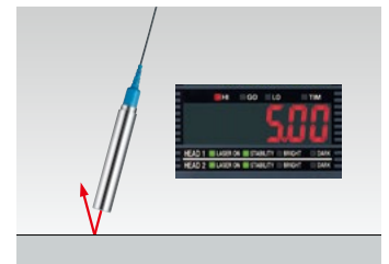
When the sensor is installed at an angle to the target: A sufficient amount of reflected light may not be returned to the sensor.
