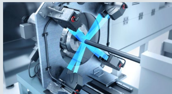
360° cable surface inspection
