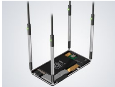
Smartphone chassis flatness inspection
