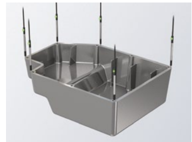
Oil pan flatness measurement
